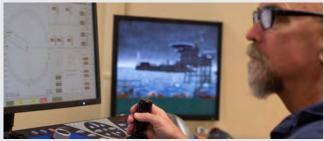
**DP SIMULATOR** allows for The Nautical Institute approved Dynamic Positioning training focused on operational procedures for adverse events, which are too complex and dangerous to train at sea
