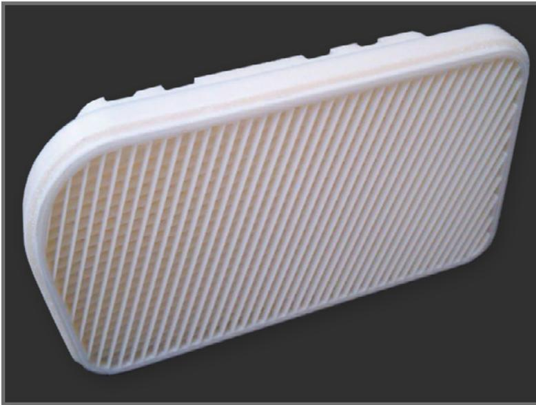
*FDM paper pulp tool with sparse fill to enable vacuum forming*
