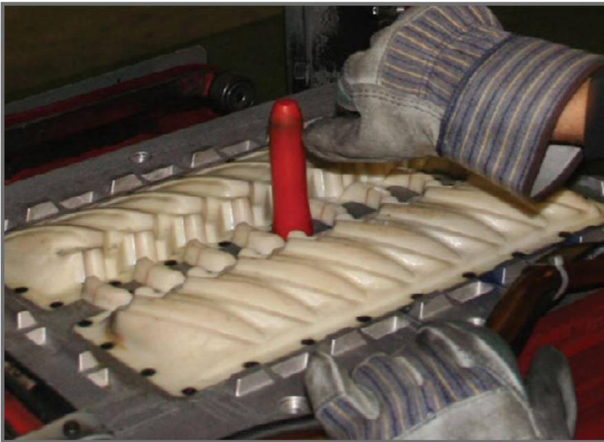
*Matchplate with FDM insert in molding machine*
